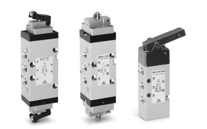
The particular mechanical device allows these end-stroke valves to operate with very low actuating forces. Series 3 has been designed with a mechanical lever device which works in negative pressure. To increase sensitivity it is possible to add to the lever a steel extension with ø 3 mm.
