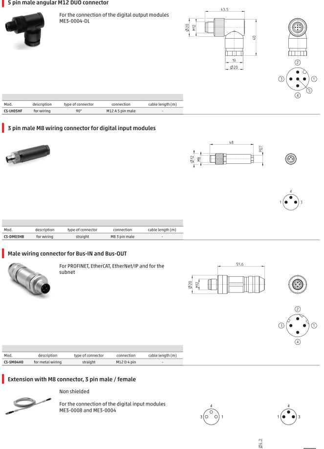
Mod. description type of connector connection L [ cable length ] (m) CS-DW03HB-C250 moulded cable straight M8 3 poli male / female 2.5 moulded cable CS-DW03HB-C500 M8 3 pin male / female straight 5
