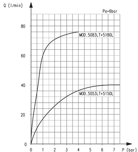
Q (l/min) = 流量 - P (bar) = 压差
