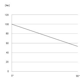
The above graph shows the torque force (in Nm) generated by a single-acting rotary actuator Series ARP during the closing action. The action starts from the 90° position and finishes at 0°. The generated torque force is at the highest at 90°, while it decreases along the stroke due to the fact that the springs get less compressed. In this case it is the springs which generates the driving force. See also the TORQUE FORCE TABLE on the following page.
