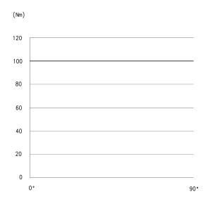
The above graph shows the torque force (in Nm) generated by a double-acting rotary actuator Series ARP during the closing action. The action starts from the 90° position and finishes at 0°. One of the features/advantages with a "rack and pinion" style rotary actuator is that the generated torque force is constant throughout the whole movement.
