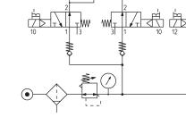
For a correct use of the rod lock Mod. RLC a pneumatic connection is recommended (as shown in the examples).
