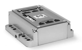
Series DRCS drives, compact and optimised in one size, are capable of controlling all Camozzi Stepper motors with two-phase and micro-stepping feed. The use of the micro-stepping control technology (up to 1/16 of a step) enables the drive to almost replicate a sinusoidal current while considerably reducing the natural resonance of the motor itself.
