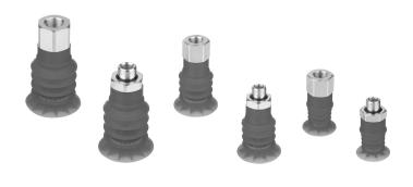
Series VPCO suction pads consist of a nipple and rubber part which are delivered assembled. Both components can be ordered separately as spare parts. These suction pads are very suitable for the handling of flexible products such as pouches and other flexible, plastic film packaging (like candy bags).
