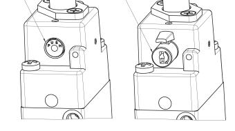
Example of solenoid valve with a bistable standard manual override.
