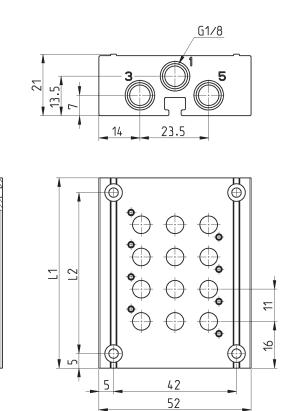
Note: the manifolds are supplied with seals and valves fixing screws.
