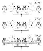
Solenoid valves available in versions with 2x3/2-way valves on
