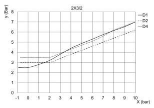
x = Inlet pressure y = Pilot pressure SOLENOID VALVES VB VERSION
