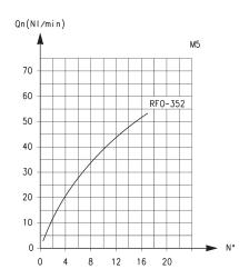
RFU 452-M5: flow from 2  $\rightarrow$  1 needle type OPEN = 55 Nl/min CLOSED = 41 Nl/min
