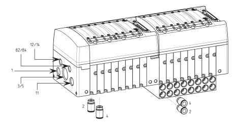
\* It is possible to connect the following fittings, supplied with O-ring: 6512-4-1/8-M 6512-6-1/8-M 6512-8-1/8-M
