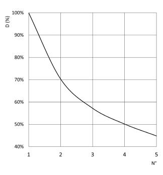
$N^\circ$  = number of valves in manifold configuration D(%) = relative percentage decay of the maximum flow rate Note: the air inlet is only from one side, in case it should be on the right and on the left, only consider the positions as from 1  $\div$  3.
