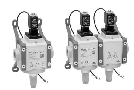
Series MX SAFEMAX solenoid valves are equipped with an integrated sensor that detects the position of the spool and enables to quickly exhaust the system in case of emergency. The sensor is in ON state (closed contact) with the valve in closing position, system exhaust. The single channel valve is classified in category 2 and can reach Performance level D. The double channel valve is classified in category 4 and can reach Performance level E.
