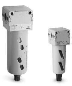
Series MC filters are available with ports G1/4, G3/8 and G1/2. Bowls are made of metal with a transparent sight glass and have a condensate drain valve which can provide either a manual or semi-automatic function.
