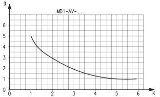
Pressurisation times as to the number of turns of the regulation screw, with downstream volume of 5 litres. A = 5 turns - B = 4 turns - C = 3 turns - D = 2 turns - E = 1 turn. K = number of turns of the regulation screw required to obtain the required pressurisation time with an inlet pressure of 6 bar. Variations of the inlet pressure can cause deviations of the pressure time by  $\pm$  20%. K = t/V where: V = volume of the downstream system in litres; t = desired pressuring time in seconds.
