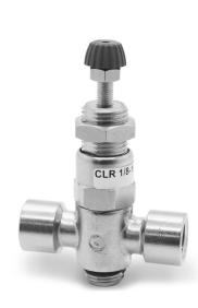
Series CLR micro pressure regulators are available with G1/8 and G1/4 connections. A piston with or without relieving and VS function (by-pass valve) has been incorporated into its design. The body is in brass, while the connection fitting is in technopolymer which guarantees maximum lightness. They can be supplied with or without banjo and can be console mounted.
