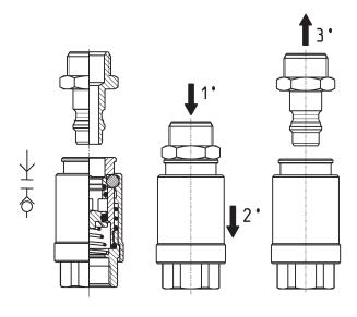
The female release couplings are designed to avoid accidental uncoupling. In fact uncoupling can only occur by pressing the male coupling inwards  $(1^\circ)$ , then the nut of the female coupling  $(2^\circ)$  and finally pull the male coupling outwards  $(3^\circ)$ .
