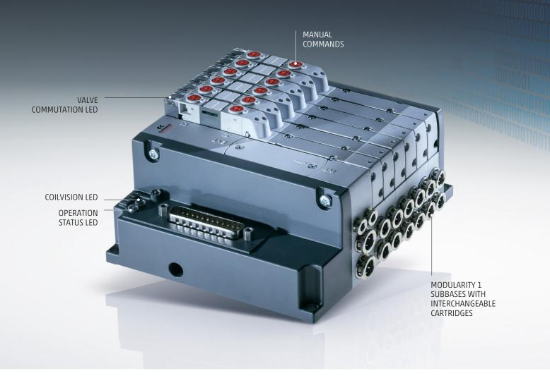
Series D is a new valve island equipped with COILVISION technology which monitors and predicts the impact of wear on the efficiency of parts of each solenoid valve. COILVISION enables proactive management of performance parameters such as power consumption and coil temperature. It also transmits operational data, alarm history and health status to a PLC or through wireless LAN to an IIoT (Industrial Internet of Things) gateway and onto the Cloud.
