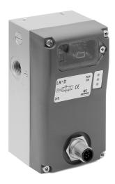
Series LR digital proportional servo valves are direct driven 3/3-way valves with a patented rotating spool system with closed loop control circuit. The electronic board is integrated into the valve's body ready to connect.
