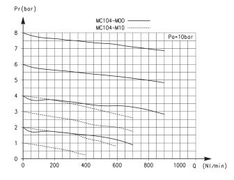
Flow diagram for model: MC104-M00
