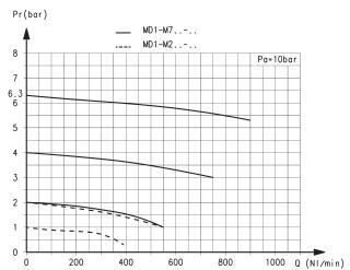
Pr = Regulated pressure (bar) Q = Flow (Nl/min)
