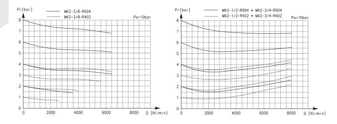
Pr = Regulated pressure (bar) Q = Flow (Nl/min)
