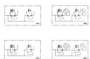
FR19 = Manifold reg. with relieving and without pressure gauge FR20 = Manifold reg. with relieving and pressure gauge FR21 = Manifold reg. without relieving or pressure gauge FR22 = Manifold reg. without relieving and with pressure gauge
