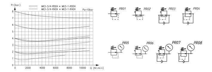
Pr = Regulated pressure (bar) Q = Flow (Nl/min)
