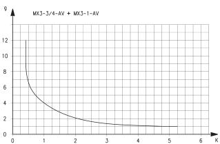
Pressurisation times as to the number of turns of the regulation screw, with downstream volume of 5 litres. A = 5 turns - B = 4 turns - C = 3 turns - D = 2 turns - E = 1 turn. K = number of turns of the regulation screw required to obtain the required pressurisation time with an inlet pressure of 6 bar. Variations of the inlet pressure can cause deviations of the pressure time by  $\pm$  20%. K = t/V where: V = volume of the downstream system in litres; t = desired pressuring time in seconds.
