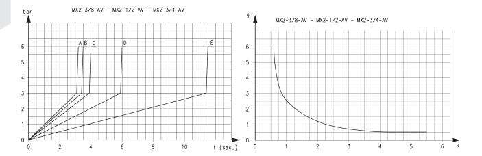
Pressurisation times as to the number of turns of the regulation screw, with downstream volume of 5 litres. A = 5 turns - B = 4 turns - C = 3 turns - D = 2 turns - E = 1 turn. K = number of turns of the regulation screw required to obtain the required pressurisation time with an inlet pressure of 6 bar. Variations of the inlet pressure can cause deviations of the pressure time by  $\pm$  20%. K = t/V where: V = volume of the downstream system in litres; t = desired pressuring time in seconds.
