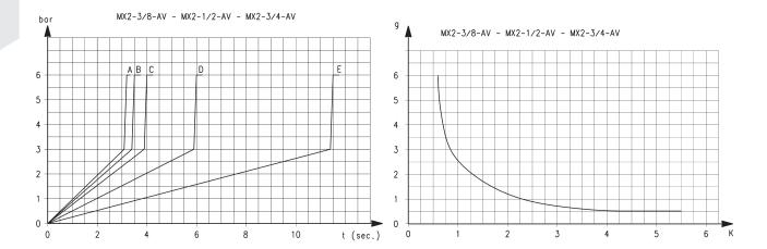
Pressurisation times as to the number of turns of the regulation screw, with downstream volume of 5 litres. A = 5 turns - B = 4 turns - C = 3 turns - D = 2 turns - E = 1 turn. K = number of turns of the regulation screw required to obtain the required pressurisation time with an inlet pressure of 6 bar. Variations of the inlet pressure can cause deviations of the pressure time by ± 20%. K = t/V where: V = volume of the downstream system in litres; t = desired pressuring time in seconds.
