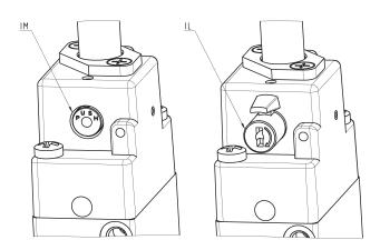
Example of solenoid monostable valve (IM) and bistable valve with a lever type manual override (IL).
