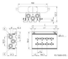
\* add - MANIFOLD PORTS (see CODING EXAMPLE) A= groove for identification label
