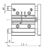
Dimensions L3 and B change according to the different strokes of QCB.
