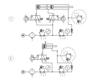
FUNCTIONING SCHEME 1: overpressure exhaust in a cylinder chamber or in a tank when the set value has been exceeded.
