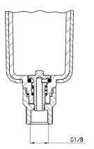
To avoid the discharge of condensate, the drain. the operator mechanism should be turned clockwise to completely close
