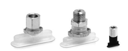
Series VTOF flat oval suction pads consist of a nipple and rubber part. The nipples are inserted directly into the rubber part. Pads size 30x10 and larger are further equipped with a special clip in order to avoid unwanted rotation during operation.
