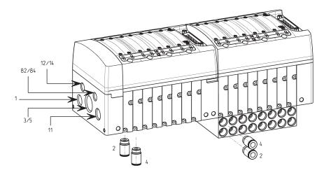
\* It is possible to connect the following fittings, supplied with 0-ring: 6512-4-1/8-M 6512-6-1/8-M 6512-8-1/8-M
