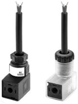
The internal rectifier circuit of the connector Mod. 125-900 allows to use solenoid valves with different AC voltage, even if the voltage indicated on the solenoid valve is DC.
