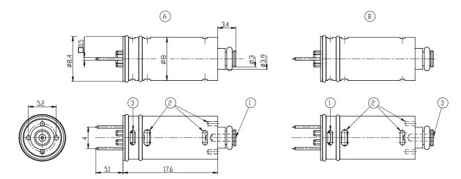
1 = ALIMENTAZIONE / INLET 2 = UTILIZZO / DUTLET 3 = SCARICO / EXHAUST A = VERSIONE 3/2 NC B = VERSIONE 3/2 NA
