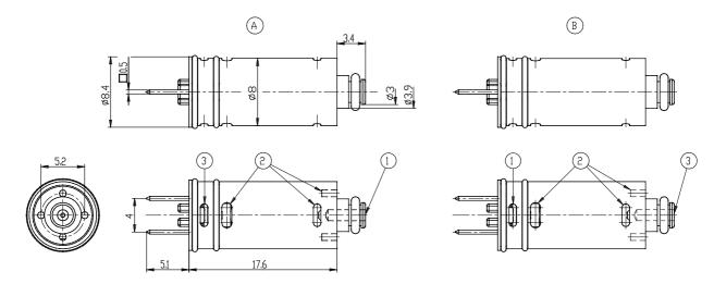
1 = ALIMENTAZIONE / INLET 2 = UTILIZZO / DUTLET 3 = SCARICO / EXHAUST A = VERSIONE 3/2 NC B = VERSIONE 3/2 NA
