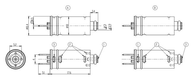
1 = ALIMENTAZIONE / INLET 2 = UTILIZZO / DUTLET 3 = SCARICO / EXHAUST A = VERSIONE 3/2 NC B = VERSIONE 3/2 NA
