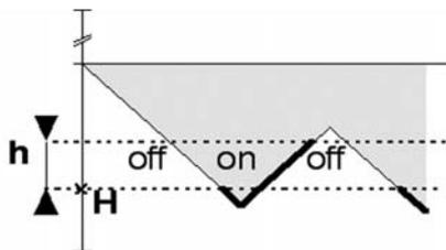
The two values which characterize the function of the switch are "Switching point H" (ex. -0,60 bar) and "Hysteresis h" (ex. 0,15 bar). With "NO" (Normally Open), at 0 bar the digital output is off.
