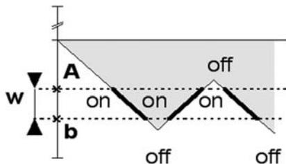
The two values which characterize the function of the switch are "Lower margin A" (ex. -0,45 bar) and "Upper margin b" (ex. -0,60 bar). With "NO" (Normally Open), at 0 bar the digital output is off.
