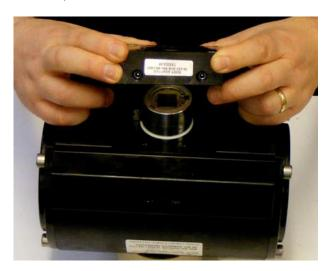
Place the cover screws and screw two of them in placed diagonally. Make sure that the gasket ("0" ring) is not damaged during the procedure.
