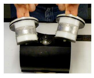
Gently pull the pinion out of the bottom of the cylinder.
