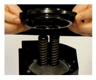
Insert the bearing into the adapter base and position it on the pinion, making sure that the holes for the adjustment screws up to the same side as the doors of the air.
