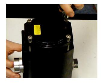
Using the appropriate tool, fix the base to the cylinder via the  $4\ \text{screws}.$
