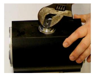
Using the appropriate tool, remove the snap ring from the top of the pinion, then remove the washer.
