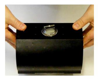
Position the actuator so that it faces you the face with the Air Ports, and the pinion cam both on the top right. Rotate the pinion 45 degrees in counterclockwise. Insert the right piston keeping the pads in front of you, while keeping the left piston rack.
