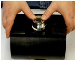
Using the appropriate tool, position the snap ring around the top of the sprocket.
