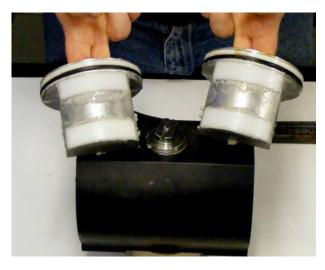
Once the pinion rack has matched up with that of the two pistons, push the latter into the actuator as far as possible.
