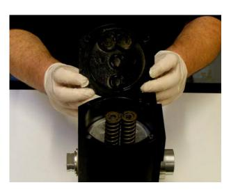
Note how the screws allow the lid to remain horizontal by being unscrewed in uniform manner.
