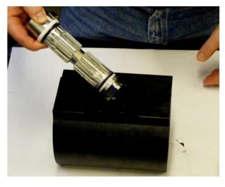
Place the "washer" on top of the pinion.
