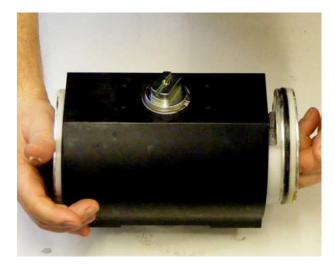
Rotate the pinion clockwise. The DD on the pinion should be at 90 degrees to the cylinder (plus a little extra), in the closed position.
