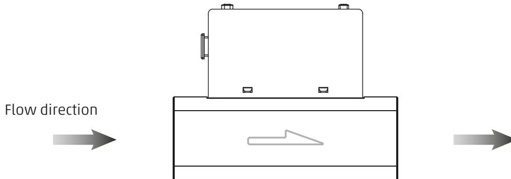
Use straight piping 8cm or longer (I.D. 9 mm or more) to connect the Piping Port (Inlet side). If straight piping is not installed, the accuracy may vary by  $\pm 2\%$  F.S.
