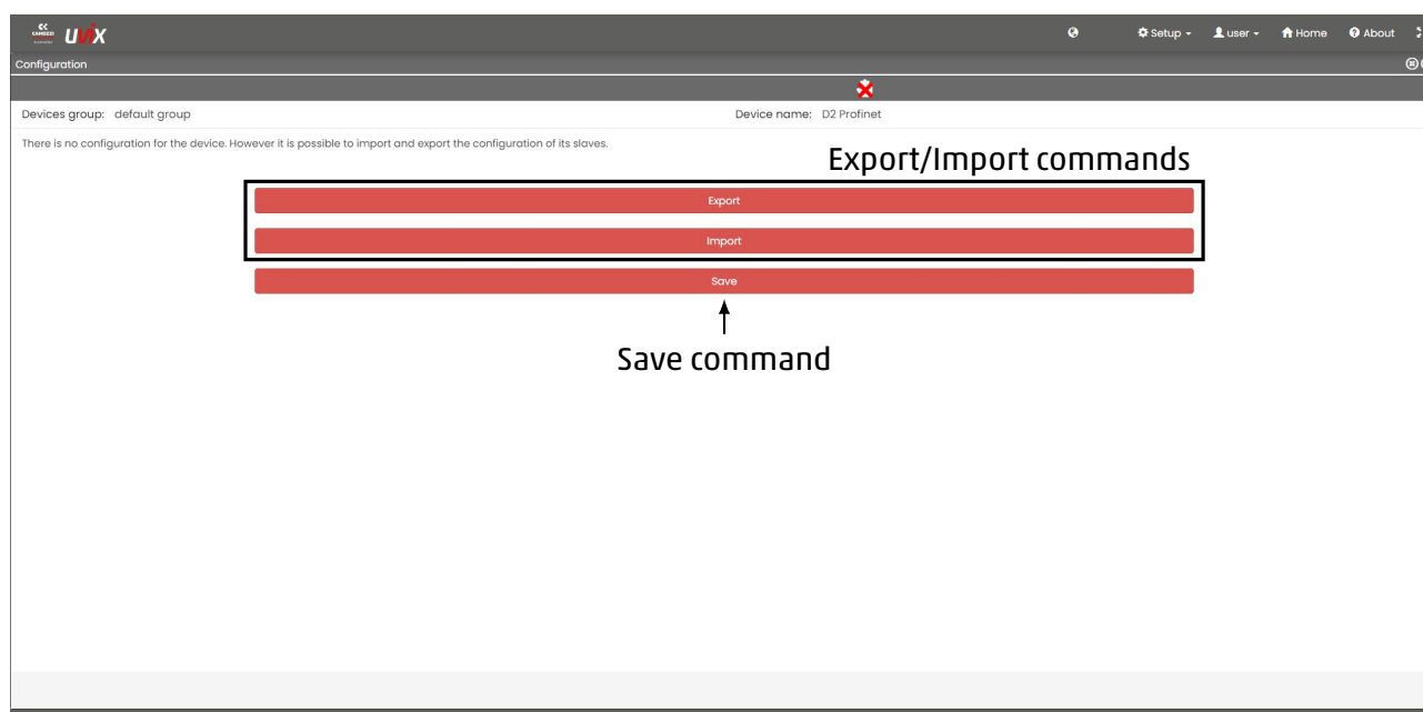
Figure 6.42: Example of Export/Import commands for a modular device
