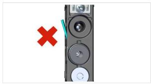
7. Check that the silencer is held tightly by pulling on the housing (hand-tight).
