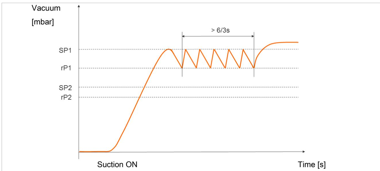
When the air saving function is activated and there is a high leakage level in the gripping system, the ejector switches between the Suction and Suction Off states very frequently. The number of valve switching procedures thus increases rapidly within a short time.
