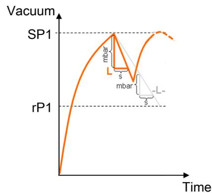
The specified value for the max. permitted leakage -L- is set in the EF menu using the parameter  $[-L-]$  or using IO-Link  $[0x006C]$ . The maximum leakage that can be set is 999 mbar/second.
