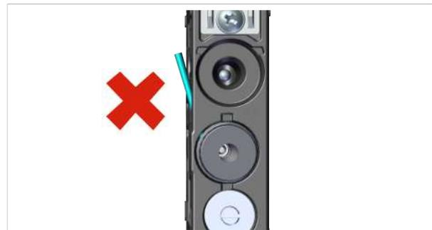
7. Check that the silencer is held tightly by pulling on the housing (hand-tight).
