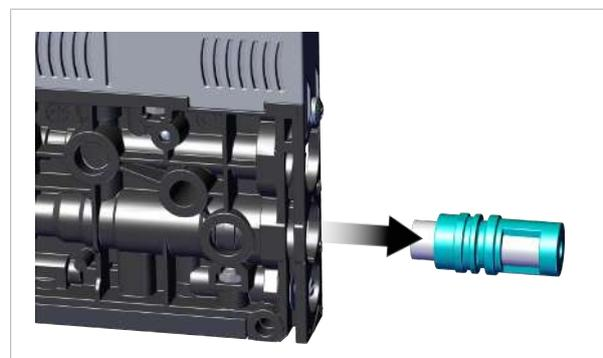
4. Pull the silencer insert out of the housing and dispose of it.
