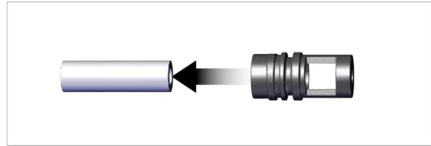
5. Insert the new silencer insert into the housing and reinstall the silencer.
