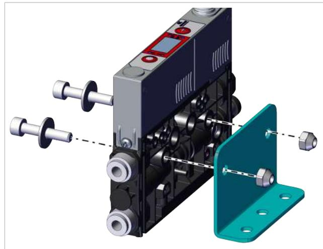
2. Loosely screw the clamps onto the bracket in the correct position.
