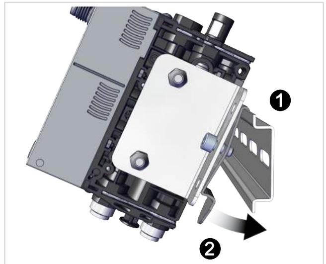
4. Tighten the screw to tighten the clamp so that the assembly is fastened to the DIN rail.
