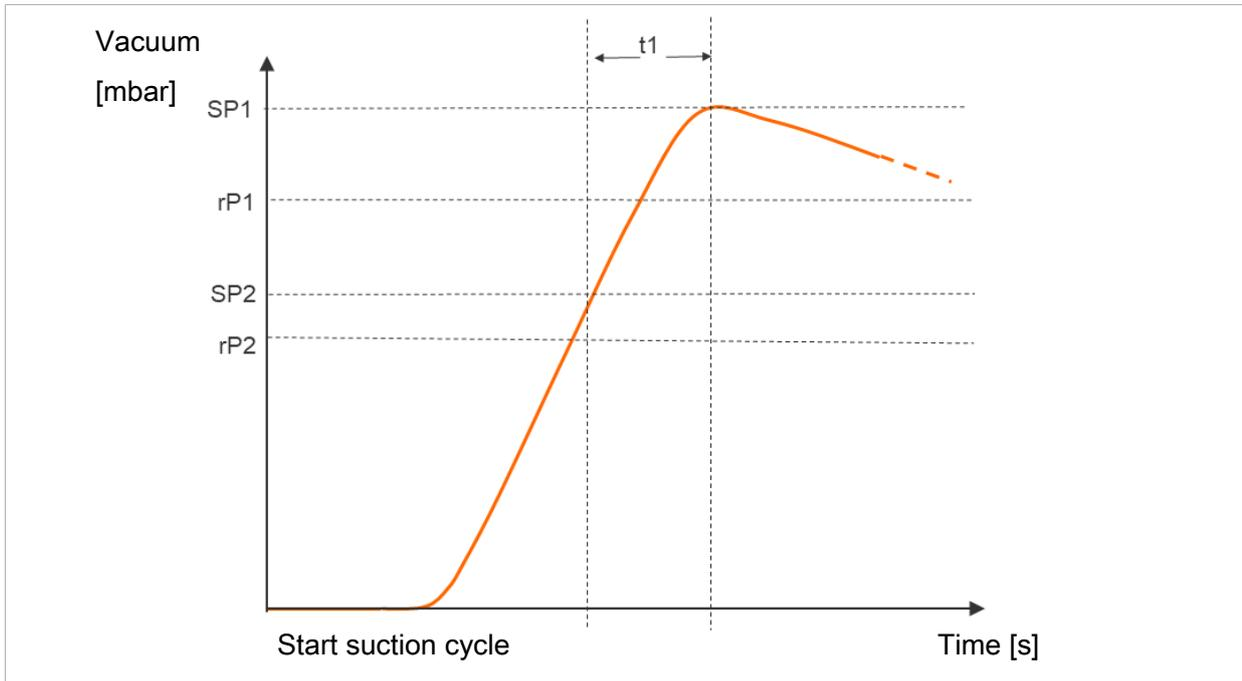
Measuring the evacuation time  $t_1$ :
