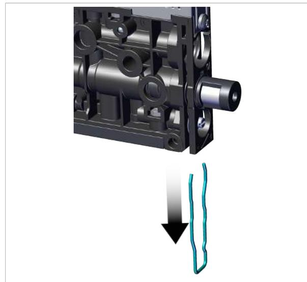
3. Then remove the silencer and silencer insert from the ejector.
