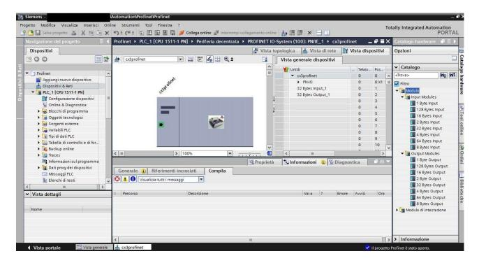
The PLC recognizes the different nodes connected to the network through the node name and then assigns them all the necessary parameters to the Ethernet communication (address, gateway, and subnet mask). The default values of these parameters are as follows: Name: empty
