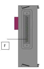
F: Sub-D female 37 poles connector for to connect the outputs
