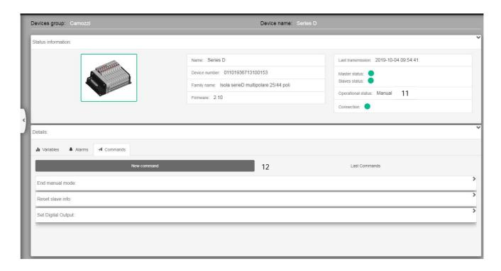
The valve island switches to manual mode (11) and the controls (12) appear on the screen
