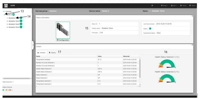
Click on the drop-down menu (13) to open the list of valves mounted on the Series D island and click on the valves (14) to display the content screen: general information (15), the health status of the individual solenoid pilot (16), the Tabs for displaying (17):
