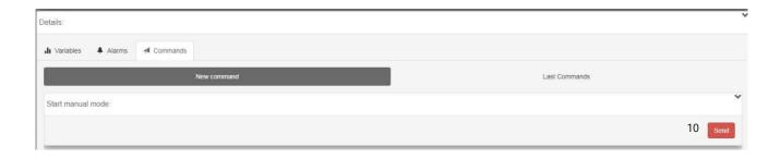
After selecting the "Tab Comands" click on the "Send" button (10) to bring the Series D valve island to "Manual" mode
