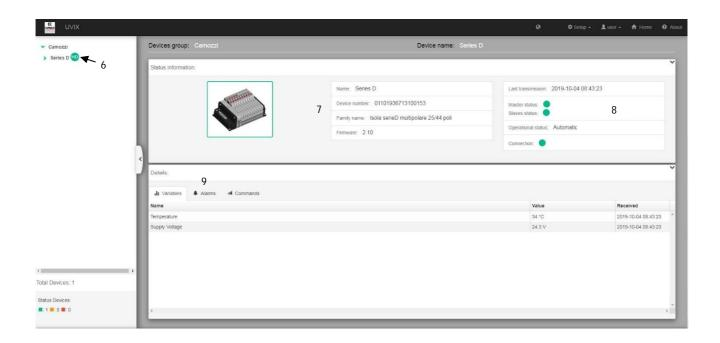
The connected Series D valve island is displayed in the list of devices (6) on the left side of the screen. Click on the name to view the relative screen with general information (7), the status of the island (8), the "tabs" (9) for viewing:
