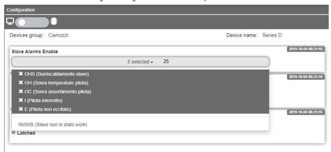
By clicking on the drop-down menu (25) it is possible to enable or disable the single alarm for the sub-base in configuration. If one of the events for which the alarm has been enabled occurs, an error message is sent.
