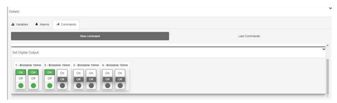
Click on the "On" and "Off" keys to pilot the single solenoid pilot and to switch the solenoid coils.
