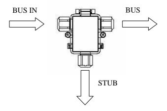
The T-derivation for the DeviceNet line has to be positioned as close as possible to the valve island Series Y in order to limit the length of the stub. In order to connect the valve island to the DeviceNet network, it is necessary to use an M12, 5 female poles connector (code CS-LF05HC for the straight connector and code CS-LR05HC for the 90° connector). In particular hard applications as regards inconveniences, it is advised to use metallic connectors.
