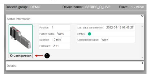
Click on the *Configuration* bottom **1** (only with *user* access) to enter in the configuration window of the single subbase/valve.
