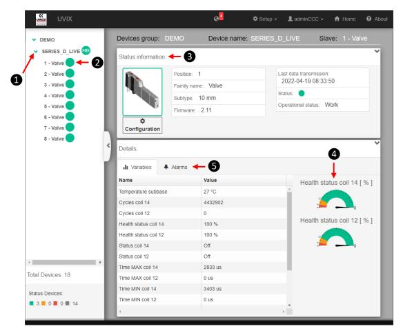
Click on the drop-down menu 1 to open the list of valves mounted on the Series D island and click on the valves 2 to display the content screen: general information 3, the health status of the individual valve pilot 4, the tabs for displaying 5:
