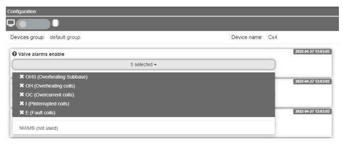
By clicking on the drop-down menu (25) it is possible to enable or disable the single alarm for the sub-base in configuration. If one of the events for which the alarm has been enabled occurs, an error message is sent. The selectable alarms are:
