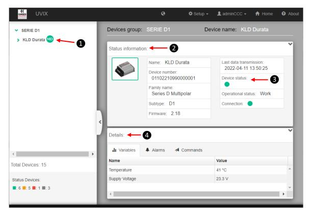
The connected Series D valve island is displayed in the list of devices 1 on the left side of the screen. Click on the name to view the relative screen with general information 2, the status of the island 3 and the tabs 4 for viewing:
