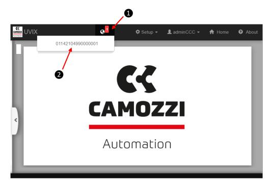
The system signals the presence of a new Series D island connected to the WLAN network.
