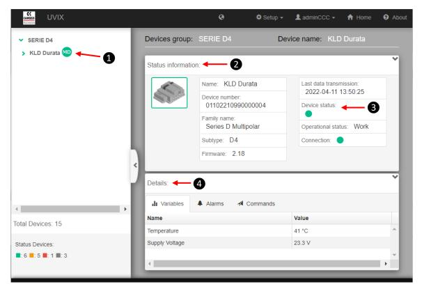
The connected Series D valve island is displayed in the list of devices ① on the left side of the screen. Click on the name to view the relative screen with general information ②, the status of the island ③ and the tabs ④ for viewing:
