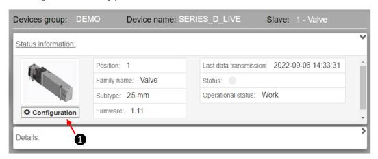
Click on the *Configuration* bottom **1** (only with *user* access) to enter in the configuration window of the single subbase/valve.
